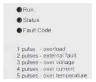
The LEDs on the front of the Variable Speed Drive indicate operating status and faults
