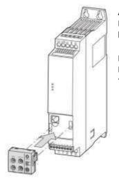
ABE is an optional module, which can be plugged onto the front of the Variable Speed Drive. It is used for simple modification of selected parameters without using a PC or keypad. All sizes of ER804 use the same module.
