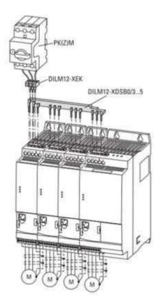
In all situations described above a direct side by side mounting of the Variable Speed Drives is permitted. This enables the use of commoning links for parallel supply of multiple drives and the use of a common protective device up to a max. current of 30 A.
